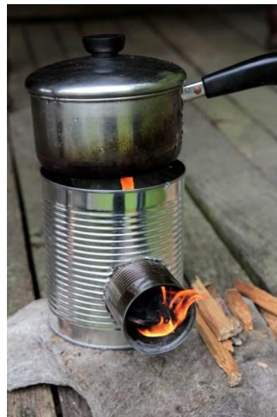
Figure 1 : Working principle of a Rocket Stove (a), and example of a rocket stove made of recycled compounds (b). Credits: (a) NokoBunva, Wikipedia contributor. (b) logcabincooking.com.
