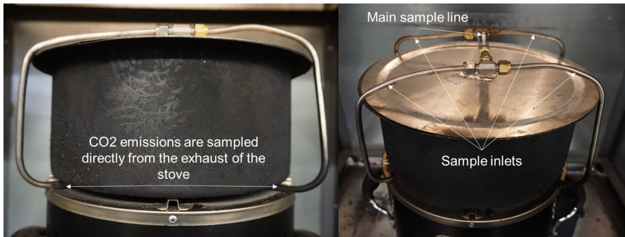
Figure 20: Illustration of the excess-air sampling rake and sample location.
