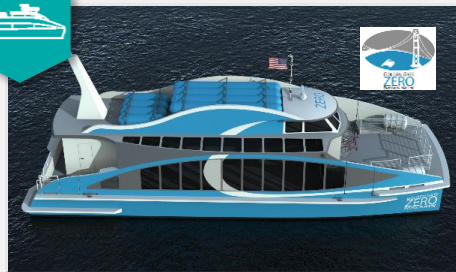
1st hydrogen vessel in the US; 70 ft hybrid hydrogen fuel cell electric catamaran (Photo: Golden Gate Zero Emission Marine)
