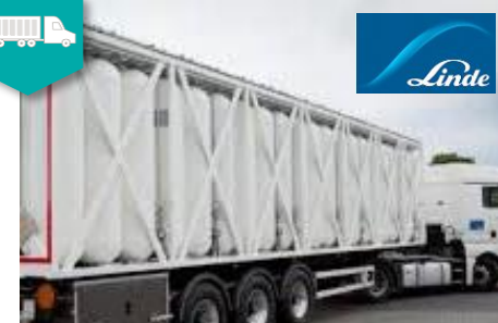
300 bar and 500 bar gas distribution modules for Linde (Photo: Linde AG)
