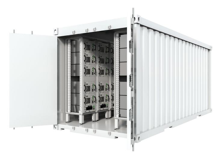
The Enapter AEM Cluster 60 is a fully assembled, ready to run and packaged electrolyser system in a 20' container. It supplies hydrogen with a rate of 30Nm<sup>3</sup>/hr at 99.999% purity. Site works are limited to the connection of vent and purge lines, water supply, hydrogen outlet piping as well as grid connections.
