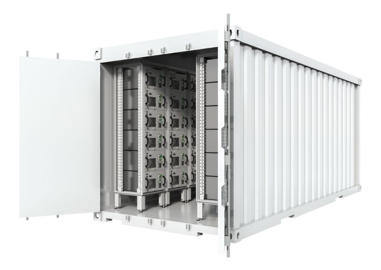
The Enapter AEM Cluster 70 is a fully assembled, ready to run and packaged electrolyser system in a 20' container. It supplies hydrogen with a rate of 36Nm³/hr at ~99.9% purity. Site works are limited to the connection of vent and purge lines, water supply, hydrogen outlet piping as well as grid connections.
