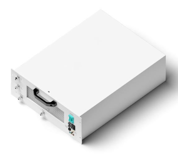
Enapter's dryer is a hybrid temperature/pressure swing adsorption system that comprises of cartridges filled with a highly adsorbent material. The dryer is maintenance-free. During operation, one cartridge catches the humidity from the hydrogen gas stream of the electrolyser, while the other cartridge is heated and regenerated. The dryer is rackmountable in a standard 19" cabinet.
