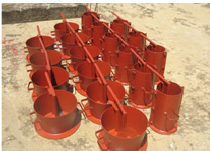
Examples of molds for Jiko Kisasa stove
