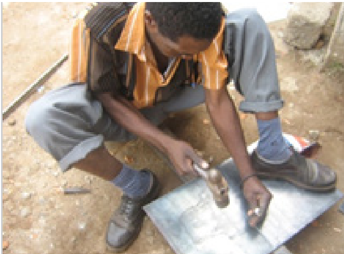
Cutting the metal plate using a cold chisel and a ball pain hammer to make the mold
