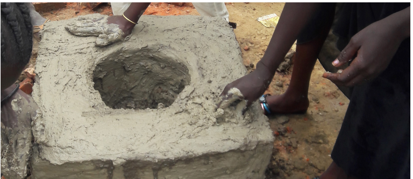
The body of the stove being built solely out of clay and cowdung
