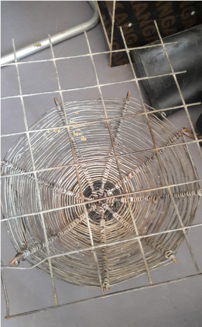
The Wire Charcoal Stove with an additional wire mesh.
