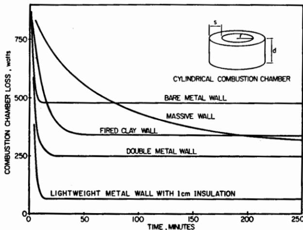
**Fig-1:** Heat loss into and through combustion chamber walls of varying material as a function of time elapsed since starting the fire. [4]
