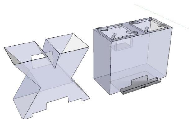
Fig-6: Three Dimensional View of Rocket Stove from Back
