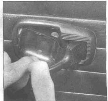
17.4 To remove the trim around the handle on 1967 and later models, pry out the recessed plastic cover and remove the Phillips screw
