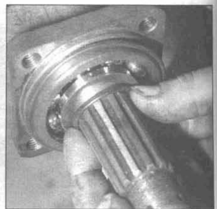
8.8c Install the small O-ring
