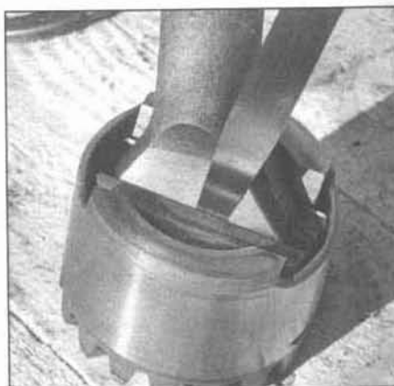
10.18b ...and, using a feeler gauge of the correct thickness, measure the clearance between the axle shaft and the fulcrum plates
