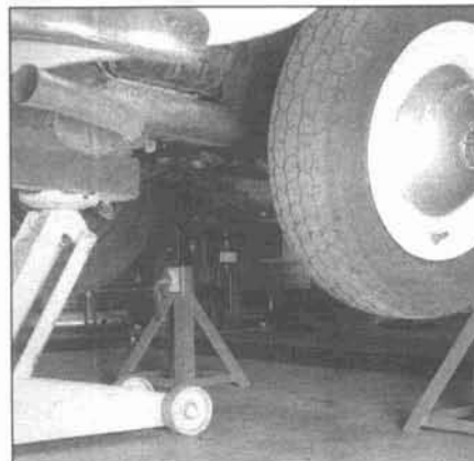
12.21 Position the jack under the center of the engine
