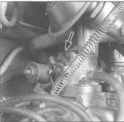
29.14 Location of the idle speed screw (arrow) on fuel-injected models
