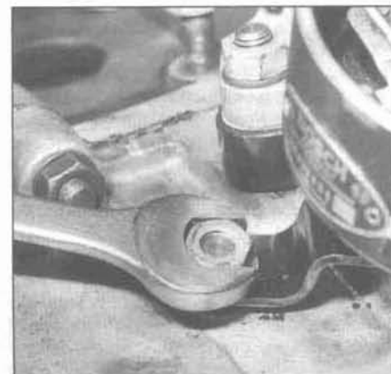
8.5 Remove the distributor hold-down nut
