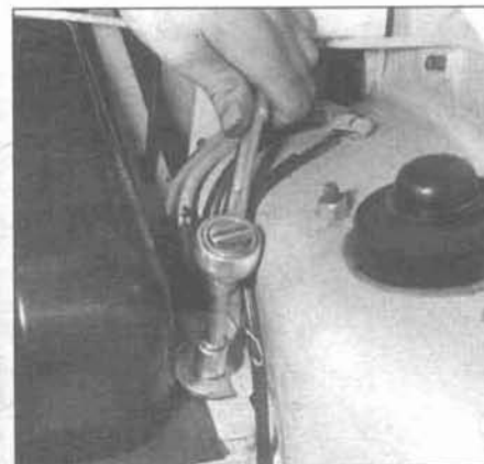
5.10 Remove the four mounting bolts and lift the fuel tank from the vehicle
