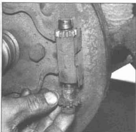
2.3j If the adjuster screws are rusted or pitted, replace them - to install the new brake shoes, reverse the previous steps
