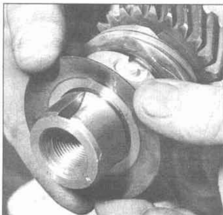
30.7 Place the oil slinger on the crankshaft with the concave face out
