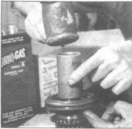
9.45c ... then drive on the hub with a suitable piece of pipe and a heavy hammer
