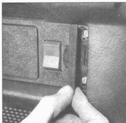
10.10 Remove these cover strips from each end of the instrument panel switch cluster
