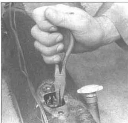
3.21 Using a pair of pliers through the hole in the tunnel for the shift lever, work the shift rod out of the coupling and through the shift rod guide bushing - keep working it forward until it's free of the bushing
