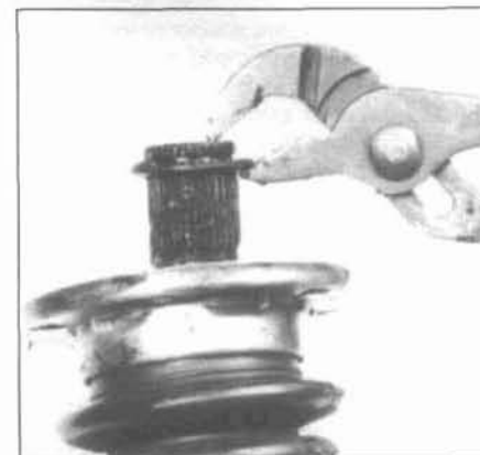
12.8a Remove the concave washer by working it up the shaft with pliers
