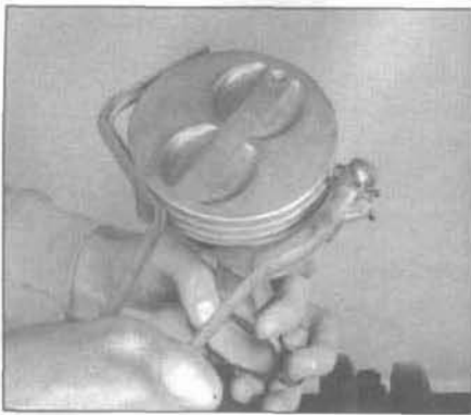
22.6a The piston ring grooves can be cleaned with a special tool, as shown here . . .
