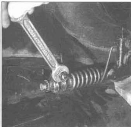
2.3a Loosen the locknut to adjust the air control ring gap - it's located between the fan housing and the firewall
