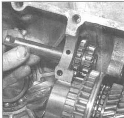
7.55 Insert the reverse gear shaft through the case, plain end first, and align the cut-out with the hole in the bearing housing
