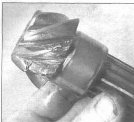
7.24 Inspect the ring and pinion gear - if either of them looks like this badly damaged pinion gear, replace both as a matched set
