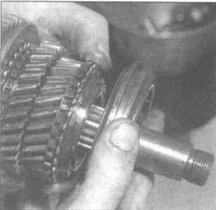
7.43 Install the third/fourth synchro assembly on the pinion shaft
