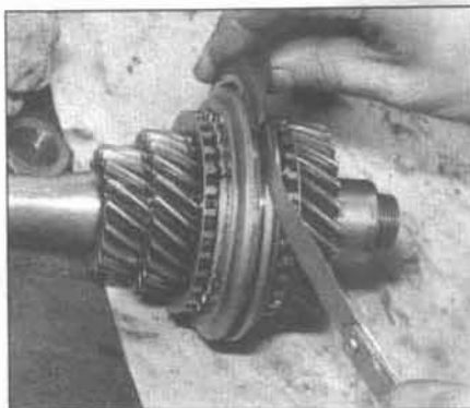
9.40 Measure the clearance between the selector fork and the groove of the synchro hub sleeve - if this clearance is excessive, the gears can jump out of mesh
