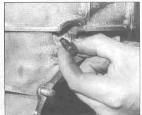
9.62c ... then insert the spacer with its slot aligned so it engages with the lock bolt screwed into the side of the case
