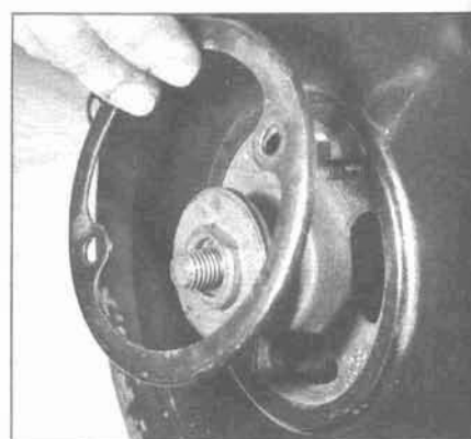
12.8b . . . the reinforcement flange and outer fan cover
