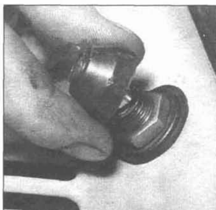
15.15a Remove the wiper shaft covers ...
