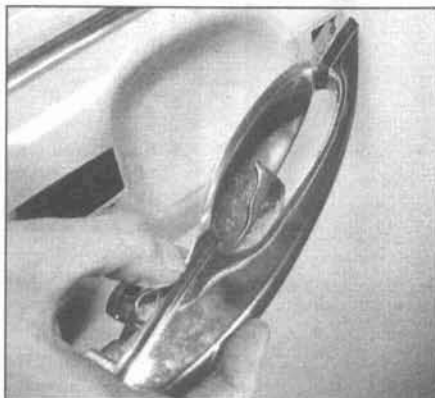
20.12b ... and remove the outside door handle and rubber seals
