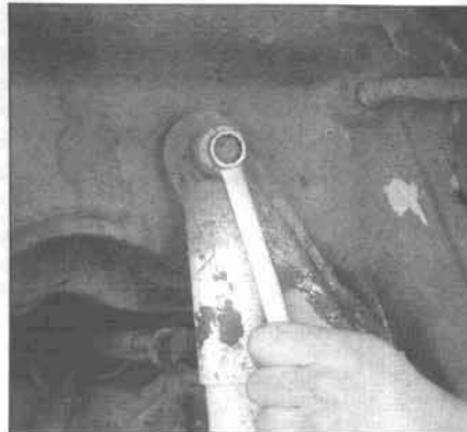
2.3a To replace a front shock absorber on a linkpin type front end, remove the upper mounting bolt . . .
