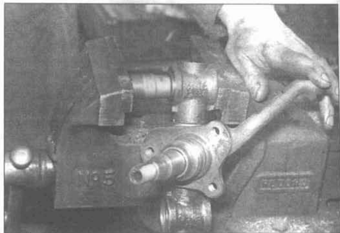
5.21b You can tap the new bushings into place with a bushing installer, socket or pipe, or you can press them into place with a vise, like this
