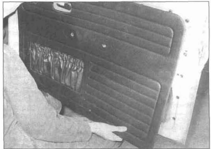
17.6a Once all the fasteners are detached, remove the door trim panel . . .
