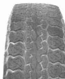
FEATHERING DUE TO MISALIGNMENT
