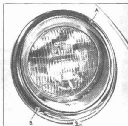
9.1a Headlight adjustment screw locations on 1966 and earlier models - screw A controls vertical adjustment, screw B controls horizontal adjustment
