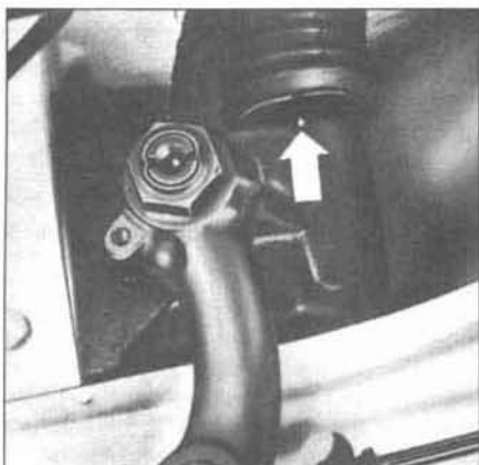
18.24 If you're installing a new boot retaining ring, center the steering and align the lug with the mark (arrow)
