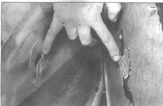
17.6c On 1972 and earlier models, you'll need to lift the door trim panel up a little so this armrest support strap on the backside of the panel clears the hook on the door - when you reinstall the panel, make sure that the strap engages the hook
