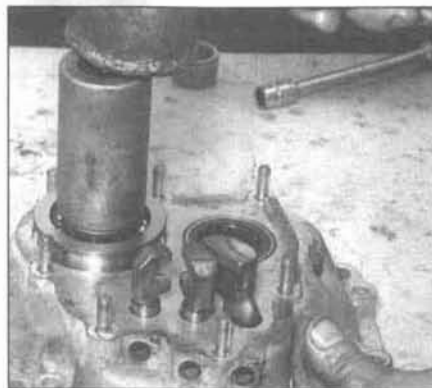
9.66b ... and tap it into place in the carrier
