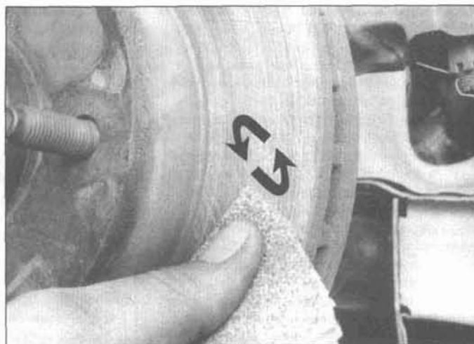
6.4b If you decide to skip machining, be sure to break the glaze on the disc surface with emery cloth or sandpaper
