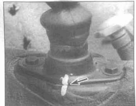
3.2 Before you loosen the bolts on the ball housing flange, mark the position of the stop plate in relation to the flange (arrow) - the plate must be properly adjusted at installation, or you'll have shifting problems
