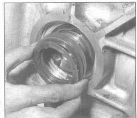
36.2 Three shims are used to set crankshaft endplay
