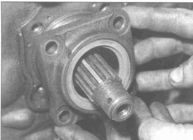
8.12 Be careful when you install the bearing cover, or you could easily damage the seal lip on the axle shaft splines
