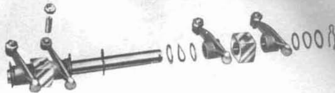
3.6a 1965 and earlier rocker arm assembly - exploded view
