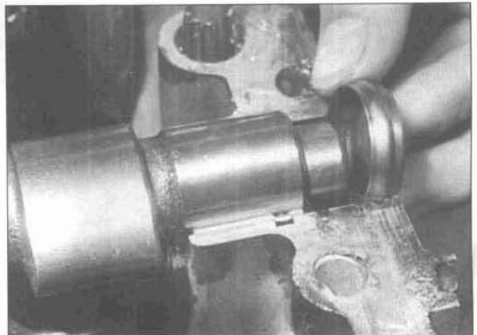
32.11 Install the circular camshaft plug
