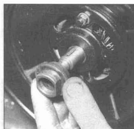
12.7b ... and slide the hub off
