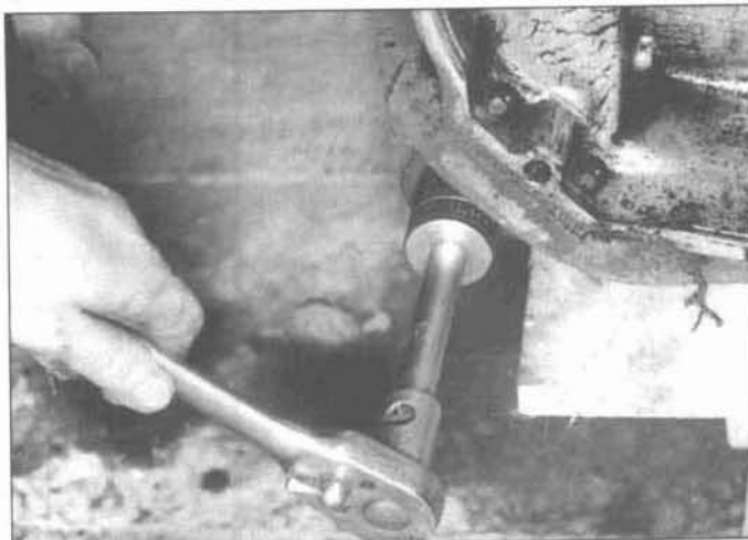
5.19 Remove the transaxle carrier bolts
