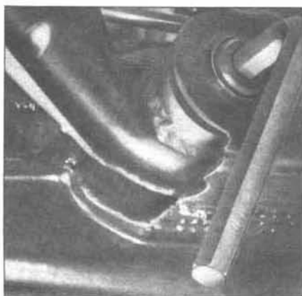
15.9 Remove the Allen pivot bolt from the front end of the diagonal arm
