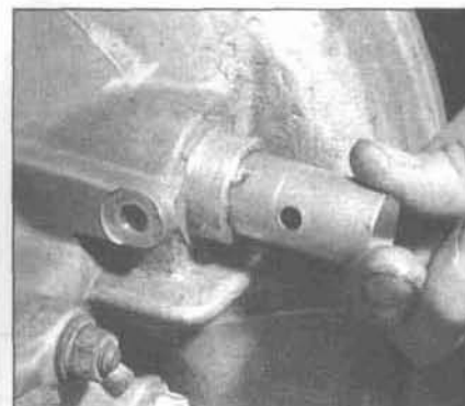
6.12 When you install the bushing, make sure the hole in the bushing is aligned with the hole in the transaxle case for the lock bolt
