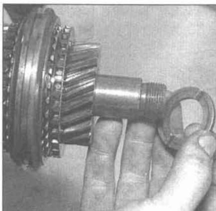
7.47 Install the thrust washer on the pinion shaft - note that the grooves in the thrust washer face the gear
