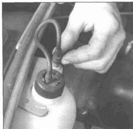
4.8 Detach the hose and remove the washer fluid filler cap
