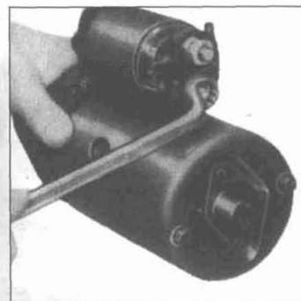
17.3 Remove the nut and the electrical strap
