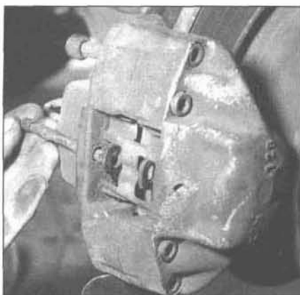
4.6 Before you remove the pad spreader spring, make sure you note how it's installed
