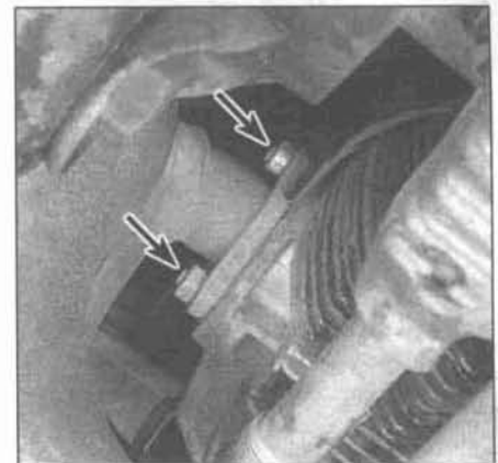
5.7 Remove the nuts (arrows) from the cylinder head studs
