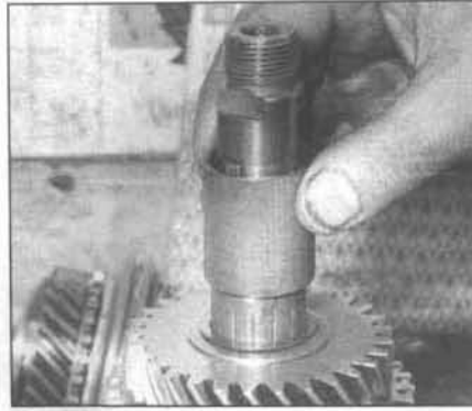
9.57c ... and install the spacer sleeve on top of the washer
