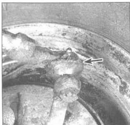
11.9 Check the balljoint boots for damage
