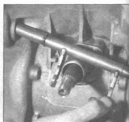
6.7 To remove the release shaft, slide it back to the right and down at the same time (don't remove that snap-ring you see on the shaft - it serves as a stop to prevent the shaft from backing out of its right bushing)
