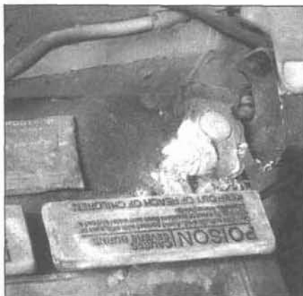
6.6a Battery terminal corrosion usually appears as light, fluffy powder
