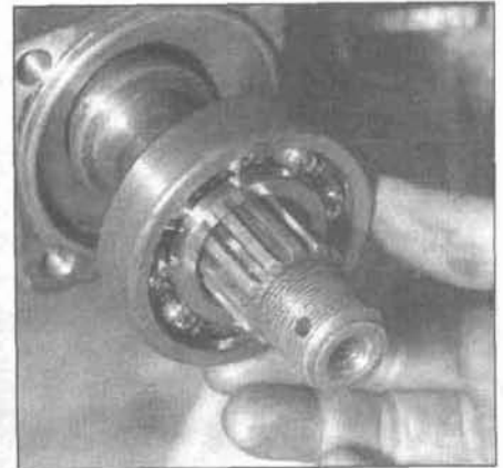
8.7 Install the rear wheel bearing
