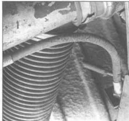
8.1 If you find a brake hose that looks like this - dried and cracked - replace it immediately!
