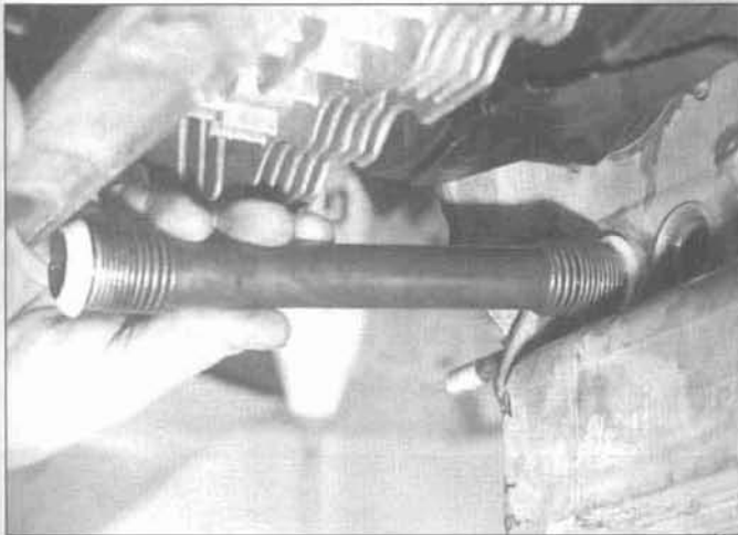
35.3 Position the pushrod tubes between the head and crankcase
