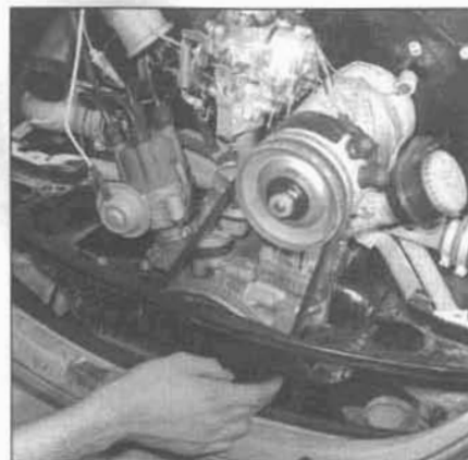
12.11c . . . and detach the rear cover
