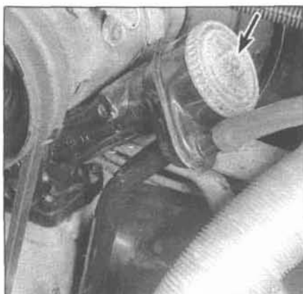
4.6 The oil filler cap is on the right (passenger's) side of the generator/alternator
