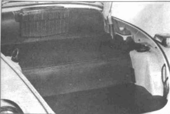
6.3 Remove the upper luggage compartment liner
