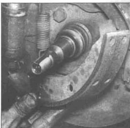
2.3h . . . then pull the front end out of the slot in the wheel cylinder, remove the front return spring and the upper shoe
