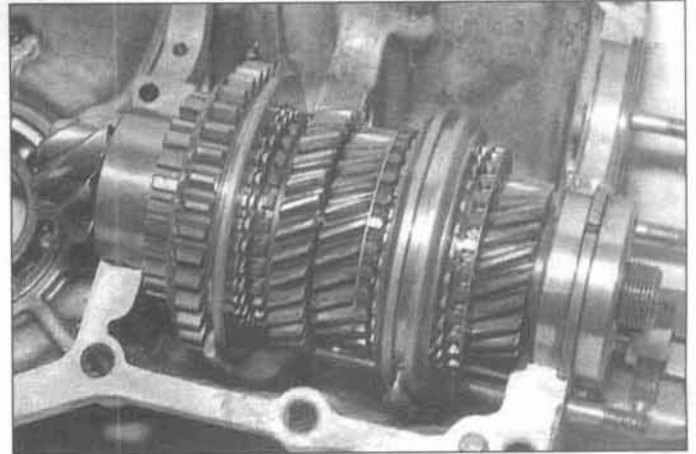
7.57b . . . verify that both synchro hub outer sleeves are in the central (neutral) position on their hubs and engage each gear to ensure that the sleeves mesh correctly
