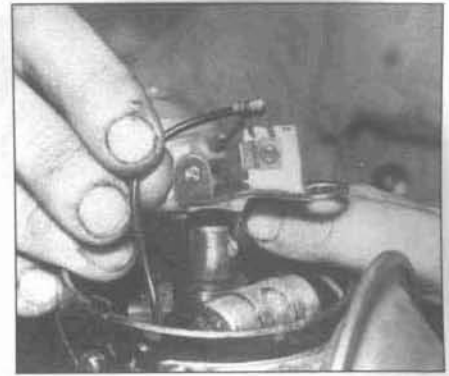
27.5b On some early models, the wire connector is attached with a screw
