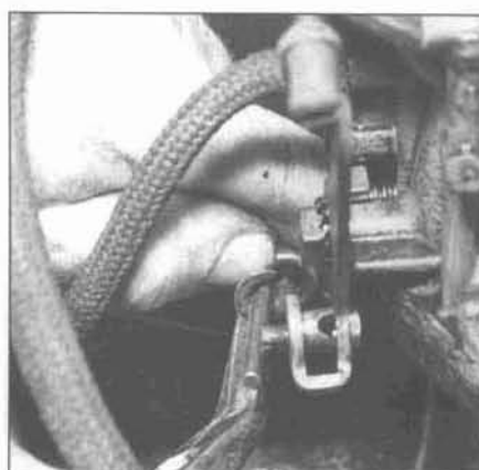
8.2b ... then remove the retaining clip (be careful not to lose the clamp screw assembly on the throttle lever)
