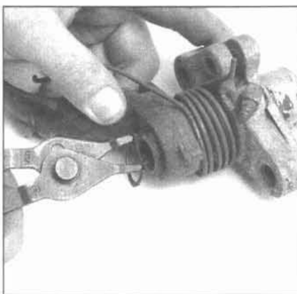
3.10 Remove the snap-ring that holds the brake pedal to the pedal cluster mount
