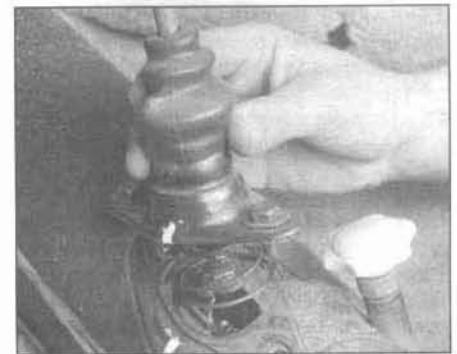
3.4 Remove the shift lever, ball housing, rubber boot and spring as a unit
