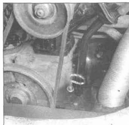
4.2 The engine oil dipstick is located below the generator/alternator
