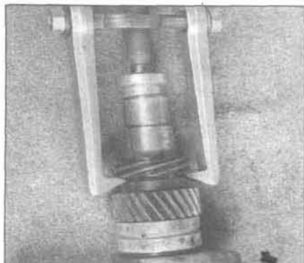
23.13 Use a puller to remove the gears
