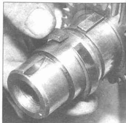
30.3 Slip the spacer in place
