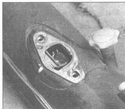
3.9 Make sure the stop plate is installed with the tab(s) facing the same way they were before removal
