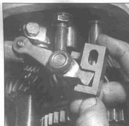
9.74a Install the selector pad and relay lever for reverse gear onto the rail . . .
