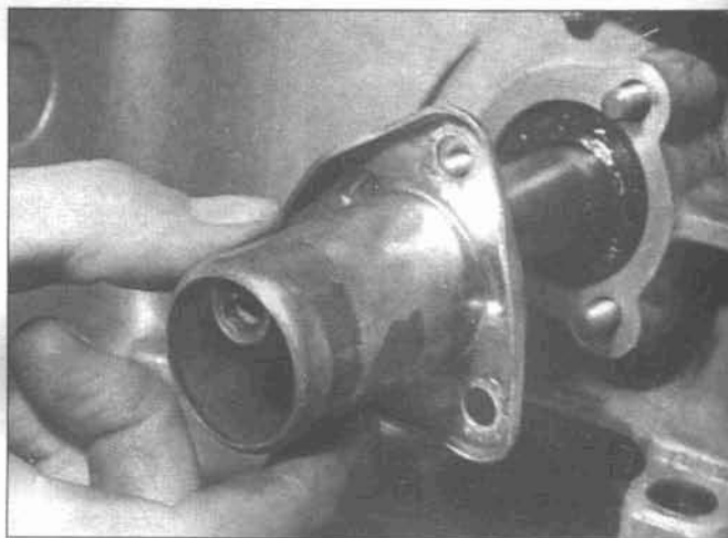
9.87d On later units, install the sleeve over the input shaft extension
