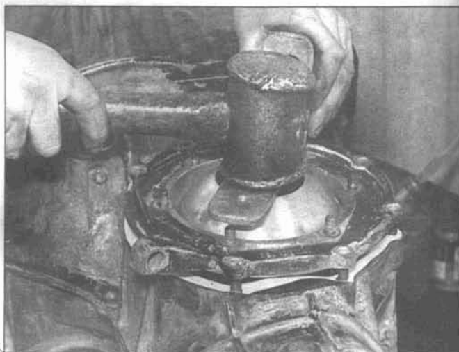
9.98b Carefully tap the left bearing side cover down onto the differential - don't use the retaining nuts to draw it down or you may crack the cover
