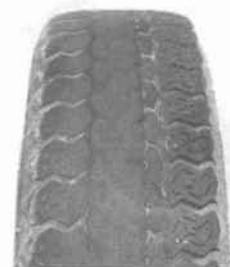
INCORRECT TOE-IN OR EXTREME CAMBER
