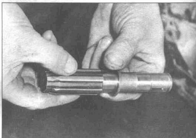
9.64a Slide the spacer ring over the shaft so that it butts against the splined section of the reverse gear shaft ...
