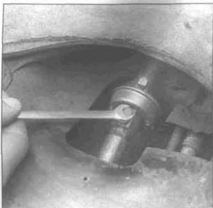
3.18a To disconnect the earlier type shift rod coupling, remove this bolt
