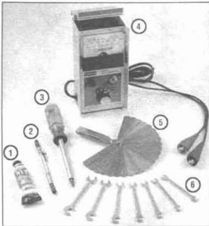
27.3 Tools and materials needed for contact point replacement and dwell angle adjustment
