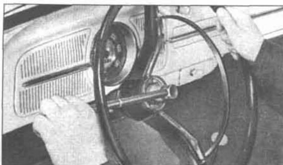
16.3 Remove the steering wheel nut and the spring washer
