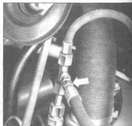
2.12 Connect a pressure gauge to the torque converter circuit to check the ATF pressure
