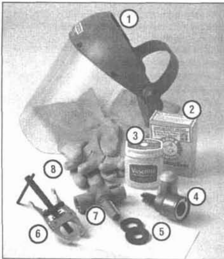
5.4a If a tire loses air on a steady basis, check the valve core first to make sure it's snug (special inexpensive wrenches are commonly available at auto parts stores)
