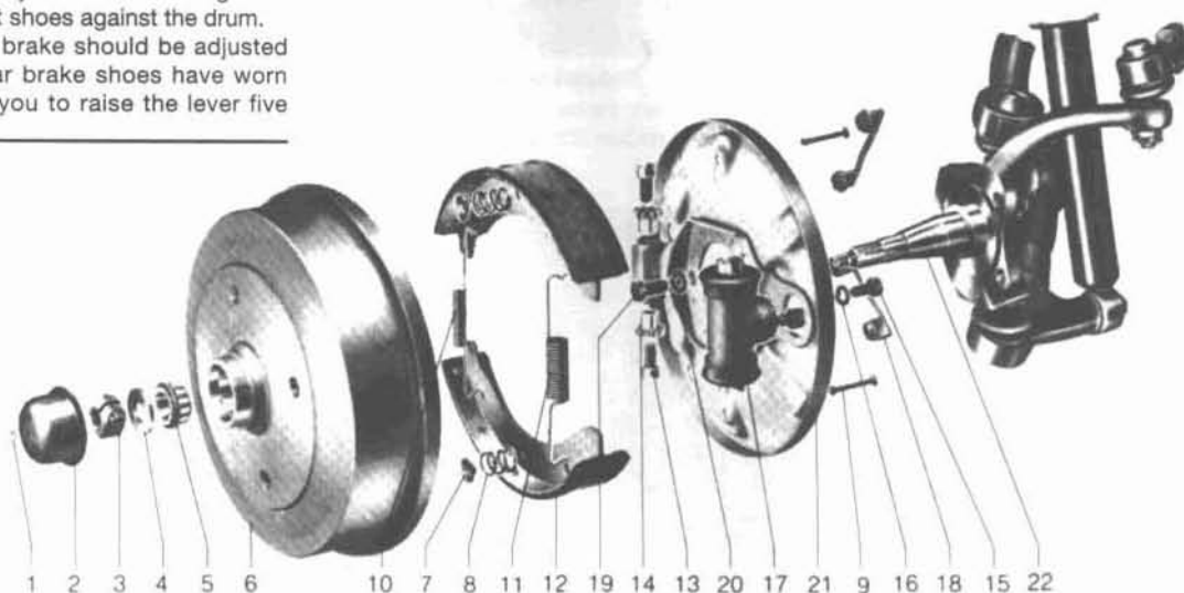
2.2a Exploded view of a typical front drum brake assembly on a torsion bar model
