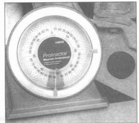
13.20 Lift the spring plate slightly to remove any freeplay, place the protractor (angle finder) on top of the spring plate and record the indicated angle
