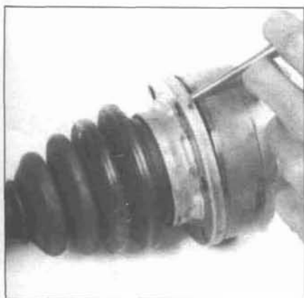
12.4 Use a hammer and punch to dislodge the boot collar from the CV joint
