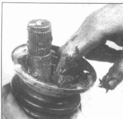
12.18 Press the grease into the boot with your fingers
