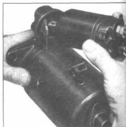
17.5 Lift the solenoid free of the starter (Bosch shown)
