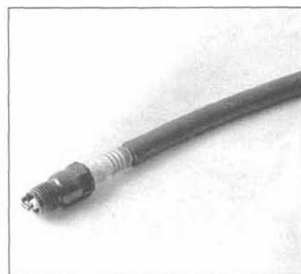
25.10 A length of 3/8-inch ID rubber hose will save time and prevent damaged threads when installing the spark plugs
