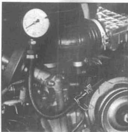
3.9 Connect the fuel pressure tester as shown - be sure to use a gauge rated for at least 50 psi
