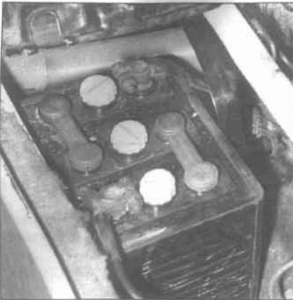
4.7a Six-volt batteries have three caps
