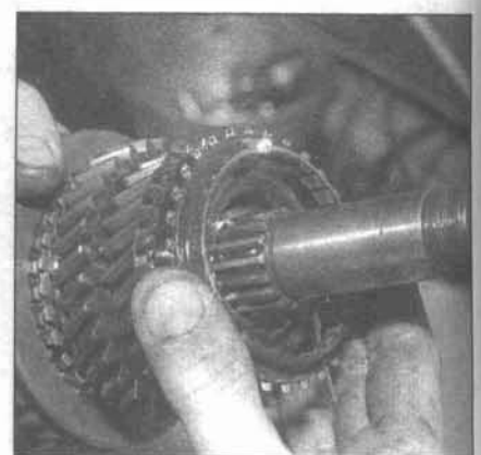
7.42b ... and the third gear synchro ring on the pinion shaft
