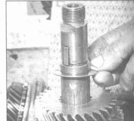
9.57a Install the dished washer on the shaft with its raised inner circumference facing toward the end of the shaft . . .
