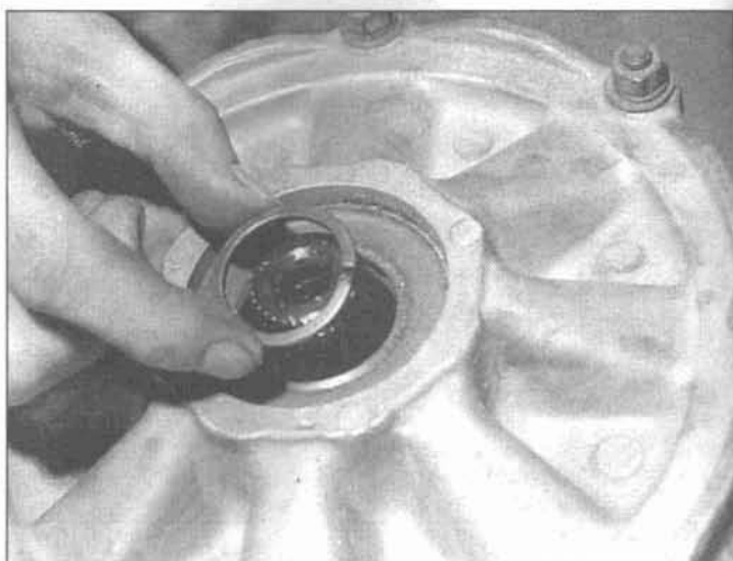
9.100a On later units with driveaxles, install the spacer ring into each side bearing cover . . .
