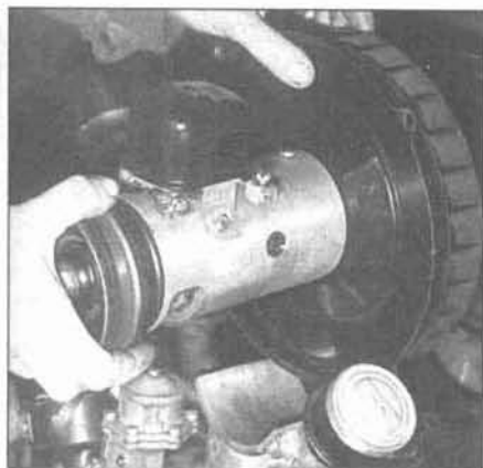
12.6 Lift the generator from the fan housing
