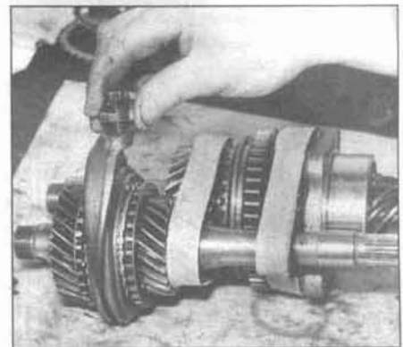
9.67 Before you install the input and pinion shafts in the gear carrier, place them side-by-side, bind them together with strong tape and place the third/fourth selector fork in position
