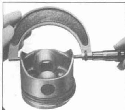
22.11 Measure the piston diameter at a 90-degree angle to the piston pin and in line with it
