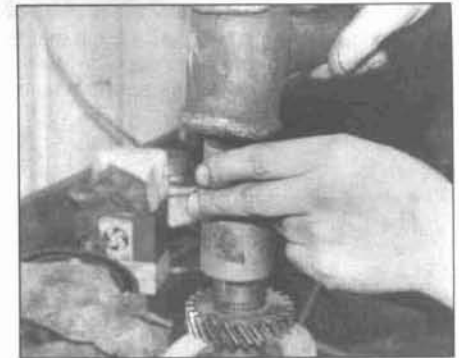
9.60 Tap the inner race for the needle roller bearing onto the pinion shaft
