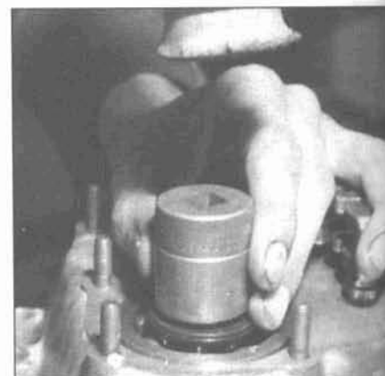
9.71 Use a socket to drive the circlip against the concave washer and pop it into the groove in the end of the input shaft on later units that don't use a nut
