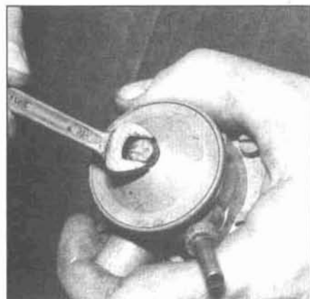
21.4a Remove the cover bolt (early model shown)
