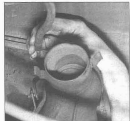
12.15 On carbureted models, disconnect the fuel line above the heat exchanger on the driver's side
